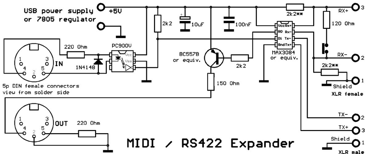
Instead of transistor BC557B every standard low frequency/low power pnp-transistor is appropriate.
