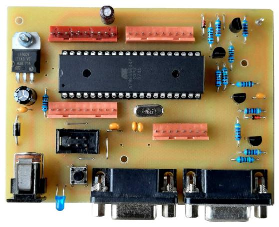
USART1 (PD2,3) is only provided at ATmega644 and ATmega1284 CPU and is intended to operate external serial equipment by Avise. This is optional and blocks other I/O at PD2,3. Very high data transfer rates cannot be expected.\_ATmega32 supports only one USART.
