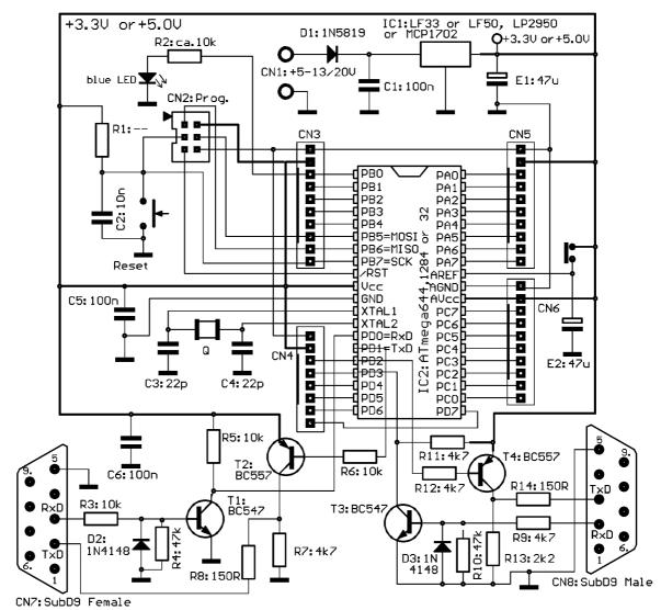
For low-freq crystals (1.84MHz) ATmega644 oscillator startup is critical. Then **for C3 and C4 check 33pf or 47pf or 68pF**. Check different oscillator start conditions (CPU flags). Sometimes another crystal works.
