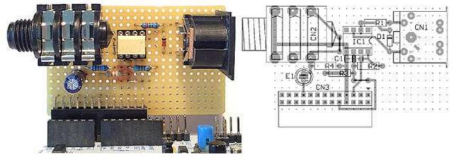
The I/O ports for USART2 are specified 5 V tolerant, for this reason R3 is not absolutely necessary. CN 3 is plugged on Nucleo CN7, pins 13-38. In the schematic assemby drawing, CN3 seems wired mirrored at a first view. But in the photo you see: the upper wires of CN3 connect the even numbered pins of the Nucleo CN7. CN3: Reichelt order.no: BL 2x13W 2,54
