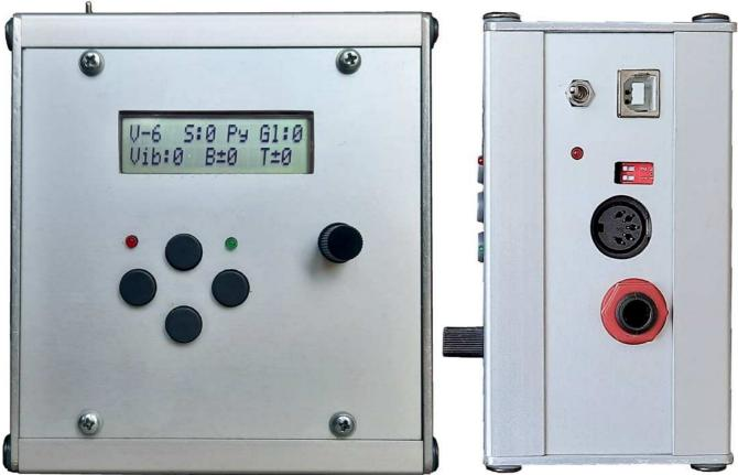
Test pins (PA15, PB7) are wired out to a 3 pin connector. Furhermore, the programming connector and reset button is extended to the front panel (for check of timing details and reprogramming while the housing is closed, not visible at this photo, bottom side of the operator panel). But this is not necessary for playing the instrument.
