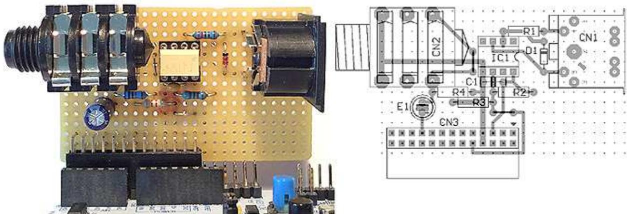
The I/O ports for USART2 are specified 5 V tolerant, for this reason R3 is not absolutely necessary. CN 3 is plugged on Nucleo CN7, pins 13-38. In the schematic assembly drawing, CN3 seems wired mirrored at a first view. But in the photo you see: the upper wires of CN3 connect the even numbered pins of the Nucleo CN7. CN3: Reichelt order.no: BL 2x13W 2,54
