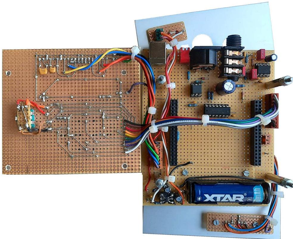
**Main board top, Operator Panel bottom.** Rear panel with Power switch and charge LED, Front panel with programmer connector, reset button expander and test pin (PA15, PB7) output for assistance of synthesiser firmware improvement while it is inside the housing. The accu+charger is provided as add-on board.
