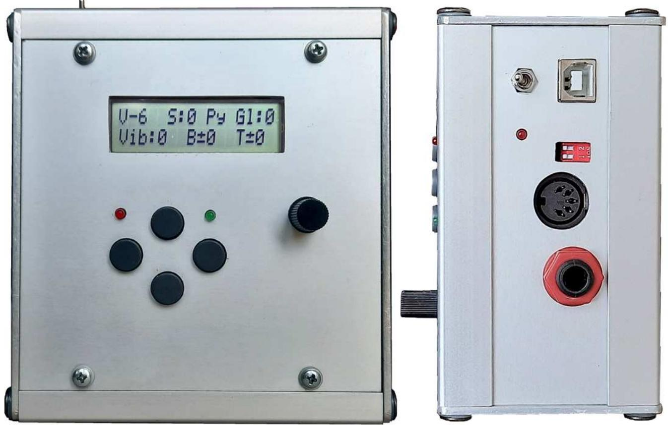
Test pins (PA15, PB7) are wired out to a 3 pin connector. Furthermore, the programming connector and reset button is extended to the front panel (for check of timing details and reprogramming while the housing is closed, not visible at this photo, bottom side of the operator panel). But this is not necessary for playing the instrument.
