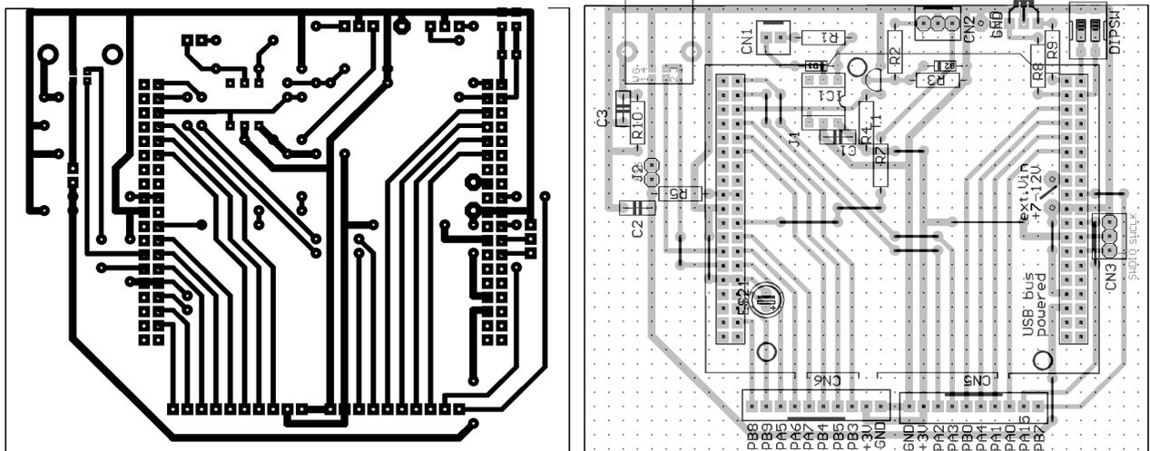
In contrast to the previous hardware version,  $V_{USB}$  is connected permanently with PA9. So it is possible (but less recommended), to supply the board with external power 7..12V DC. Due to Veroboard limited wiring resolution, the wire is put via PB2, which is HiZ input and 5V tolerant. J1 is only used for measurement of supply current. For longterm practical use it should be shorted with solder.
